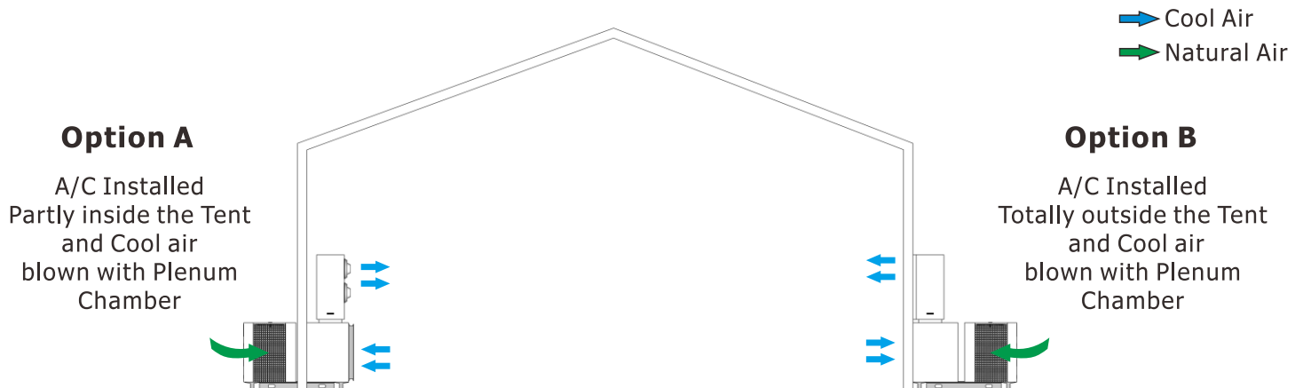
Demonstration of A/C Installed Inside and Outside the Tent
